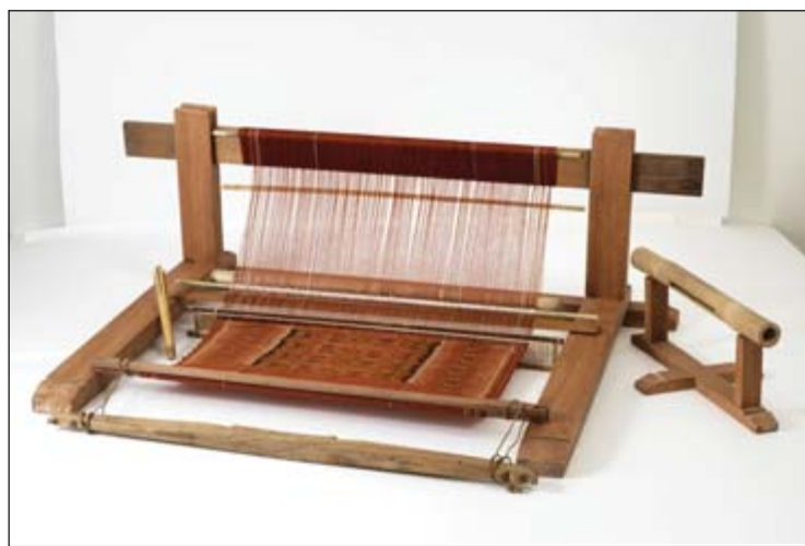
Ngurah Hendrawan and Ni Gede Diari. Cagcag (backstrap loom), comprising frame, yoke, shuttle, blade/beater, reed, lease bar, string heddle, and loom cloth. Nusa Penida, Bali, Indonesia, 2017. Wood, bamboo, cotton. Bard Graduate Center Study Collection. —Bruce White photo
